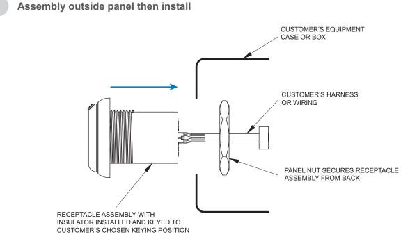
Install receptacle body then assemble inside panel
