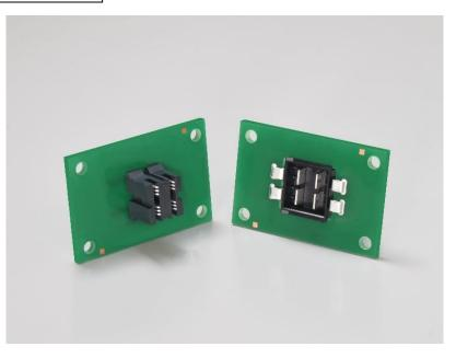
This product uses our unique floating structure, which are capable of  $\pm 0.8$ mm floating tolerance in the X and Y directions. DW11 series is a connector that can be customized with the number of terminal required for a customer application. This connector series is ideal to supply power between boards, and will cater to applications in various industrial applications.
