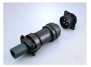
The JL10/W Series is an outdoor circular connector equipped with a bayonet style one-touch lock enabling fast mating and unmating, while providing a reliable lock when in the mated condition.
