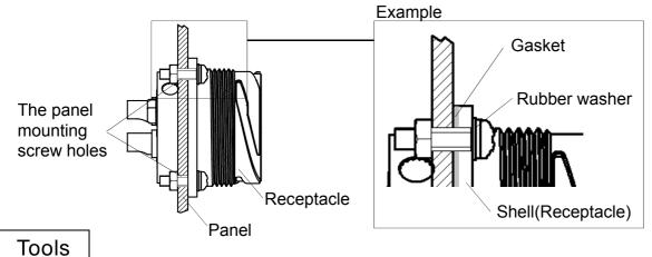
Using screw with rubber washer to prevent water ingress through the panel mounting screw holes.
