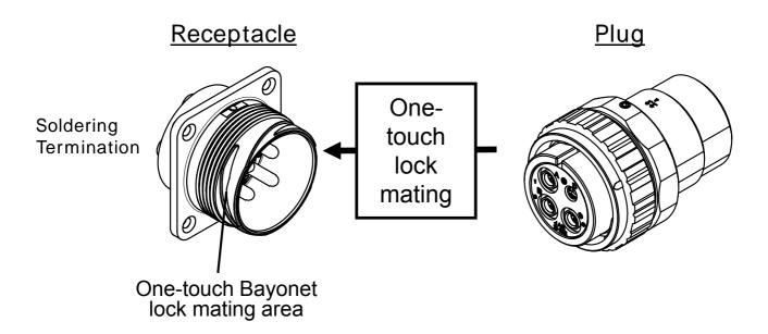
The JL10/W Series is an outdoor circular connector equipped with a bayonet style one-touch lock enabling fast mating and unmating, while providing a reliable lock when in the mated condition.
