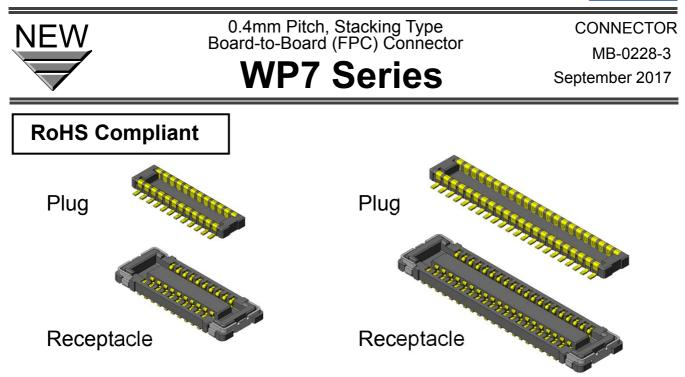
The WP7 Series is a low-profile board-to-board (FPC) connector with 0.4mm pitch spacing that is ideal for high-density mounting in slim information communication devices like mobile phones, smartphones, LCD, and notebook PC.
