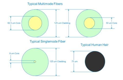
In fiber cable, light is carried down the core. The larger the core, the greater the amount of light paths or modes. In fiber cable, the light source emits photons down the fiber core. Each photon carries the same signal down the path (or mode). But only one photon is required for an optical signal to be received.
