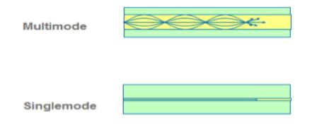
In multimode fiber, multiple photons (or modes of light) travel down the fiber core. However, in long cable runs (greater than 3000 feet [914.4 m]), multiple paths of light can cause signal distortion at the receiving end, resulting in an unclear and incomplete data transmission.
