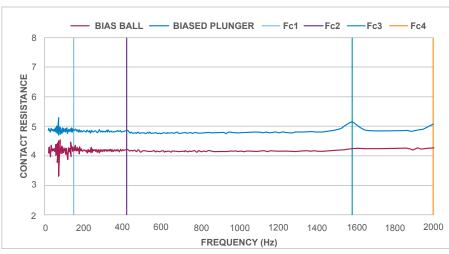
DYNAMIC CONTACT RESISTANCE DURING FREQUENCY SWEEPING: X AXIS -15G INPUT Graph 4
