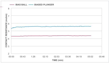
DYNAMIC CONTACT RESISTANCE AT WORST RESONANCE FREQUENCY F<sub>c</sub>=1550Hz - X-AXIS -15G Graph 6
