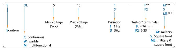
F\*\* If no terminal specification, the model is standard delivered with round pins, diameter 1.5 mm. Fast-on terminals are available in 2 dimensions: F = 4,76 mm (0,187 inch) or F = 6,35 mm (0,250 inch).
