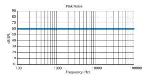
When a pink noise with a certain Vrms is sent to a speaker and the produced sound of the speaker is recorded with a microphone, the amplification response of the speaker can be showed.
